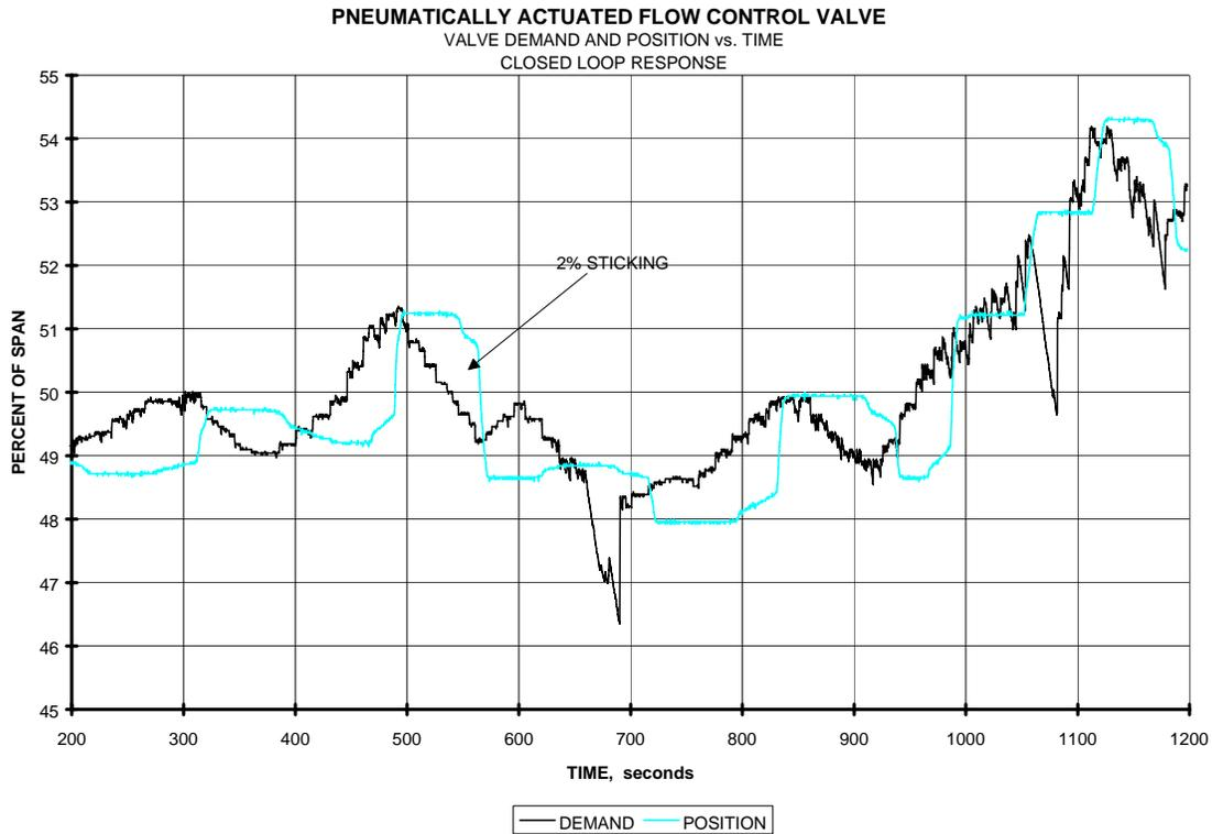
Bump testing produces a “popping” action, which allows a pneumatic actuator to more easily overcome valve stiction than when it is gradually modulated, as is characteristic of closed-loop control. Pneumatic actuator performance is, therefore, far more susceptible to the ill effects of stiction under closed-loop control conditions than under bump test conditions.
