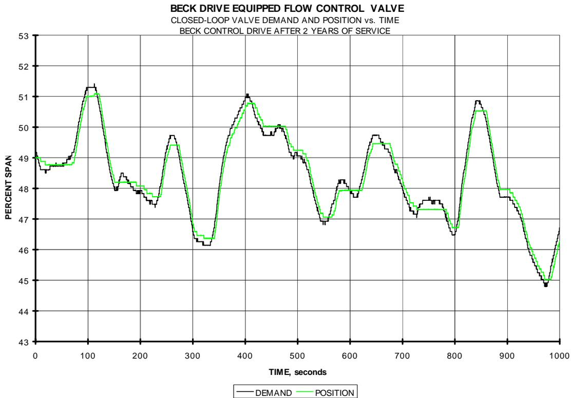
As with pneumatic actuators, the open-loop bump response of a Beck drive is not necessarily indicative of its closed-loop response; however, the reason this occurs, and
