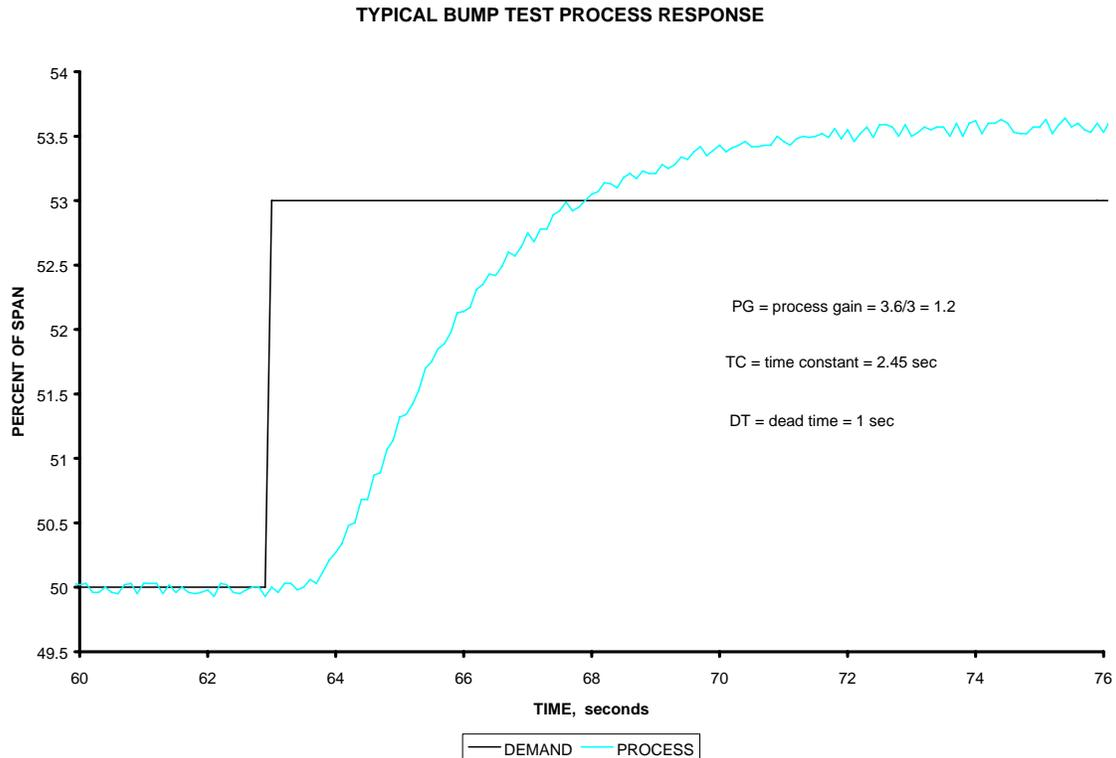
The goal of any tuning method is to establish tuning parameters that will produce optimal *closed-loop* control performance. Unfortunately, *open-loop* actuator performance is not necessarily indicative of *closed-loop* performance. Therefore, dynamics established from open-loop bump testing may not reflect the process dynamics under closed-loop conditions. This is the drawback of open-loop bump testing.
